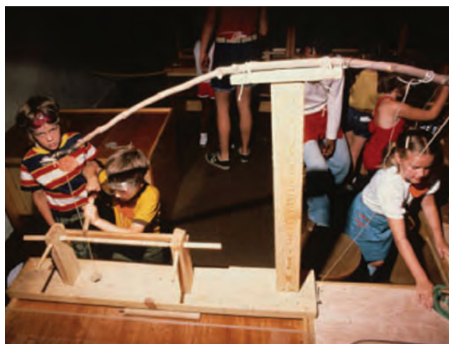
Using accessible and inexpensive materials Bernie, left, builds a pump drill—a tool that goes back thousands of years—out of a coffee can, string, and a dowel. In the Tools exhibit, right, kids use a working model of a pole lathe to shape wooden dowels.
