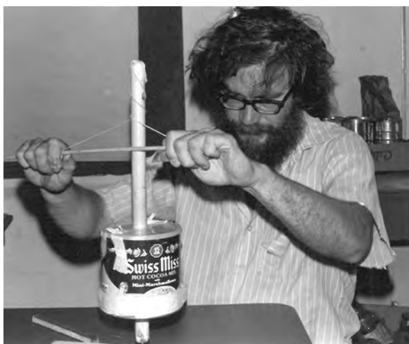
Using accessible and inexpensive materials Bernie, left, builds a pump drill—a tool that goes back thousands of years—out of a coffee can, string, and a dowel. In the Tools exhibit, right, kids use a working model of a pole lathe to shape wooden dowels.
